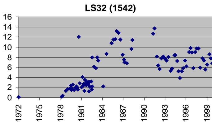
Figure 50. Southwest Sprayfield Monitor Well Nitrate Concentrations (as N, mg/L).
