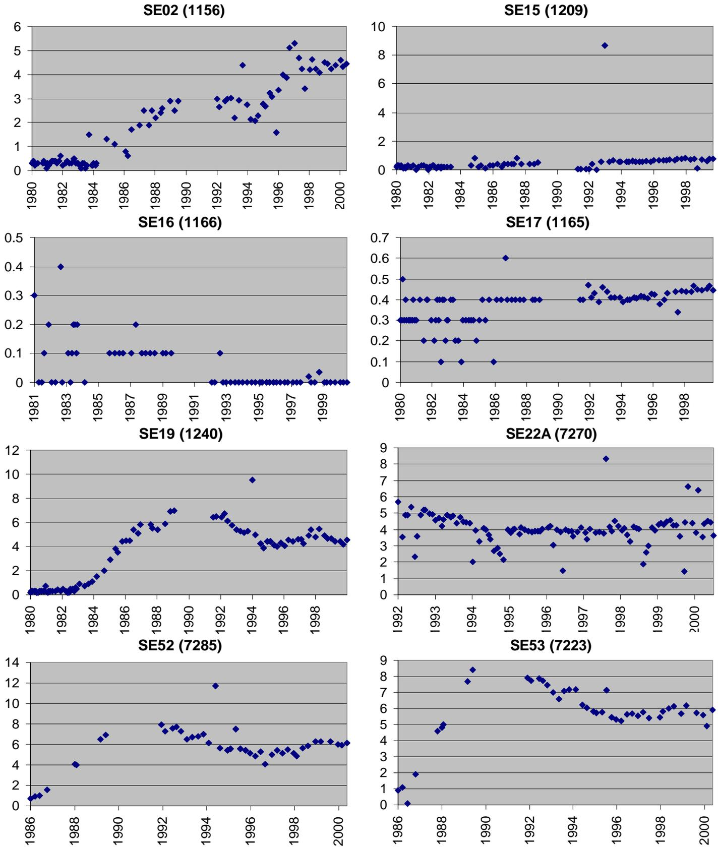
Figure 48. Southeast Sprayfield Monitor Well NO<sub>2</sub>+NO<sub>3</sub>-N Concentrations (mg/L)
