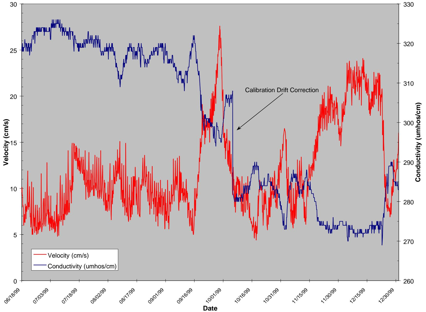
Figure 33. 1999 Wakulla Springs Velocity versus Specific Conductivity.
