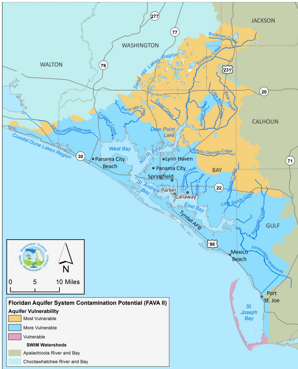
Figure C-1 Floridan Aquifer System Contamination Potential
