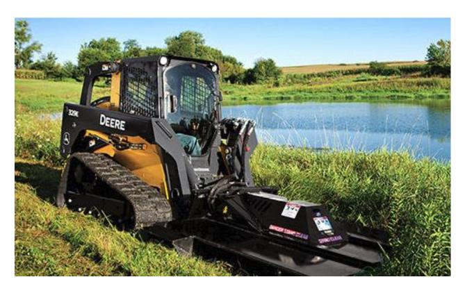
**Limb Beaver** attachment for clearing roadside vegetation, slopes, ditches. Works vertically, horizontally, and below horizontal for sloped edges.
