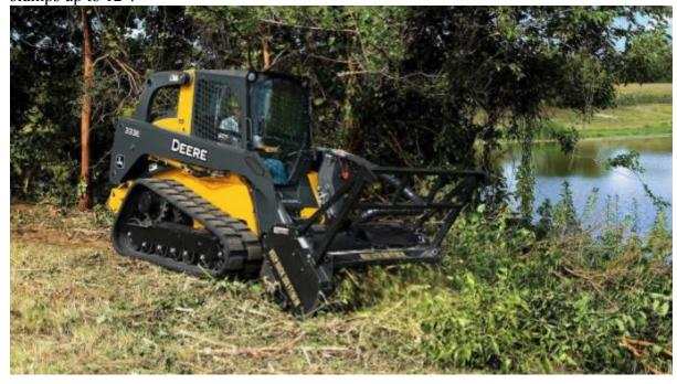
**Hydraulic Rotary Drum Mulching Head**
