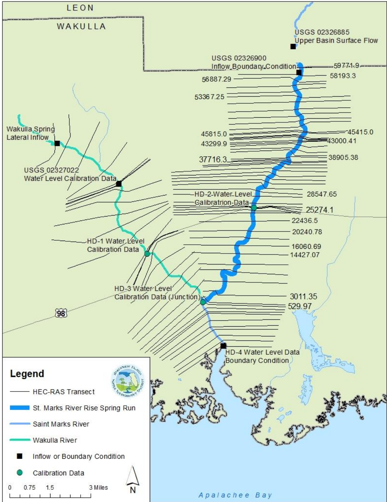
Figure 3-7: HEC-RAS Model Geometry, Boundary Conditions, and Calibration Sites
