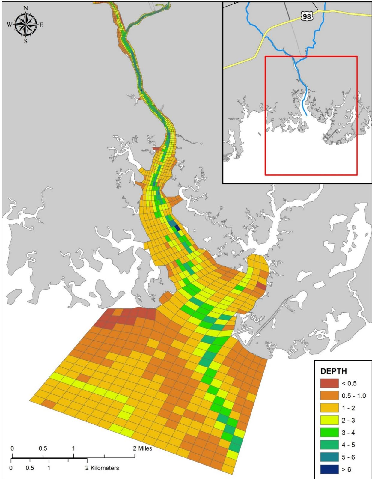
**Figure 3.** Model grid and bathymetry for the St. Marks River from the confluence downstream to the offshore boundary of the model domain. Vertical reference is NAVD88, vertical (depth) units are meters.
