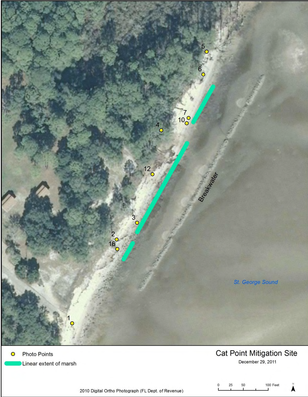
Figure 4. Aerial photograph of mitigation site with location of photographic points indicated. At the time of inspection the marsh (indicated in bluegreen) had expanded to cover nearly the entire length of the breakwater.
