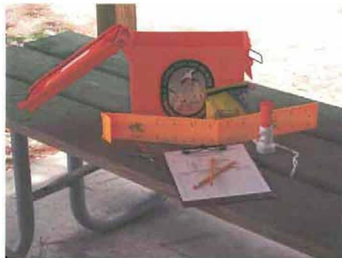
Figure 12. Creel kits are assigned to each angler, who is asked to collect species and length on each fish he/she catches. Rulers, pliers and safety equipment are also provided.
