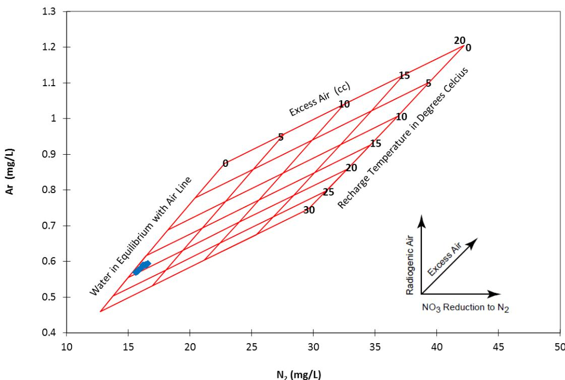
**Figure 14. Dissolved N<sub>2</sub> vs Argon Plot: Gas Concentration Normalized to Sea Level**
