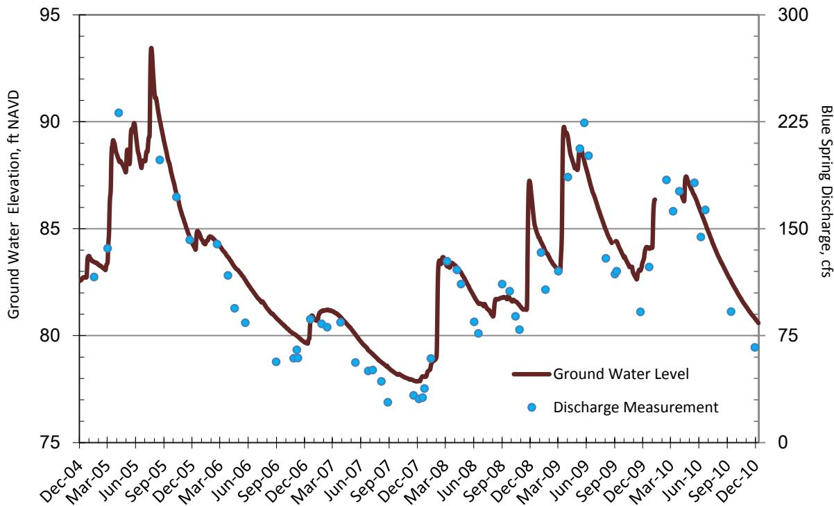
Figure 5. Discharge measurements and ground water levels measured at the Pittman well
