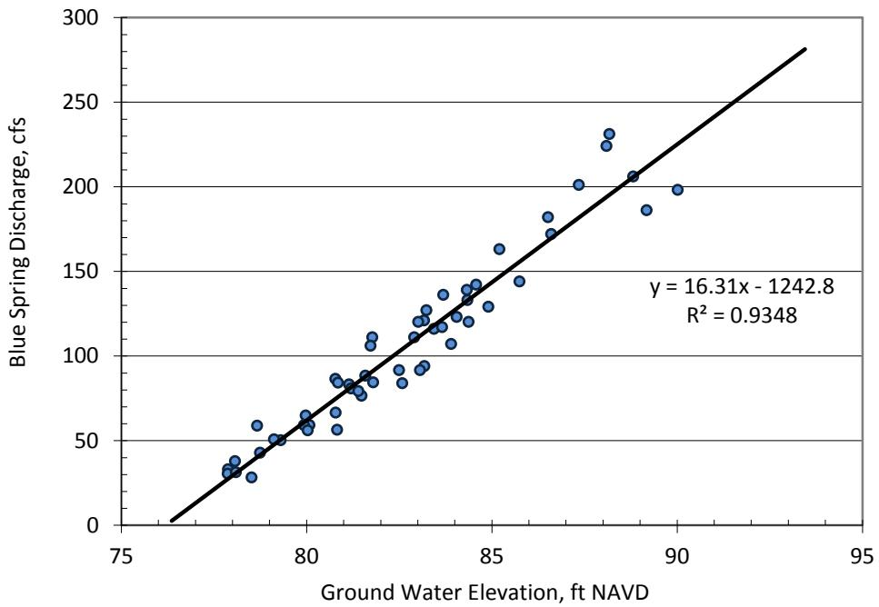
**Figure 6. Ground water level-discharge relationship for Jackson Blue Spring**
