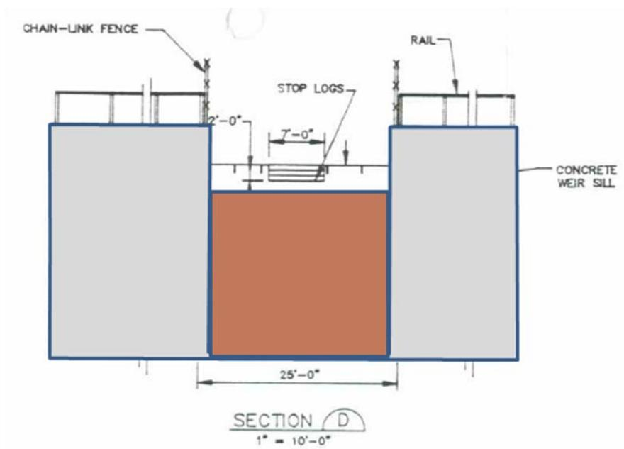
**Figure 1. Merritt's Mill Pond Outflow Control Structure**
