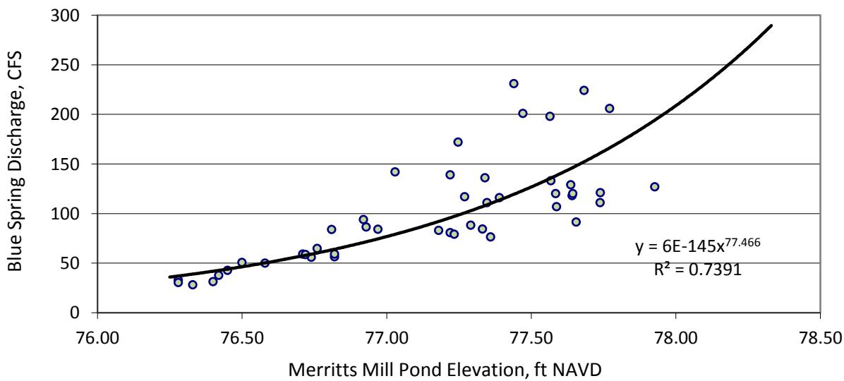
**Figure 8. Merritt's Mill Pond Elevation and Measured Spring Discharge**
