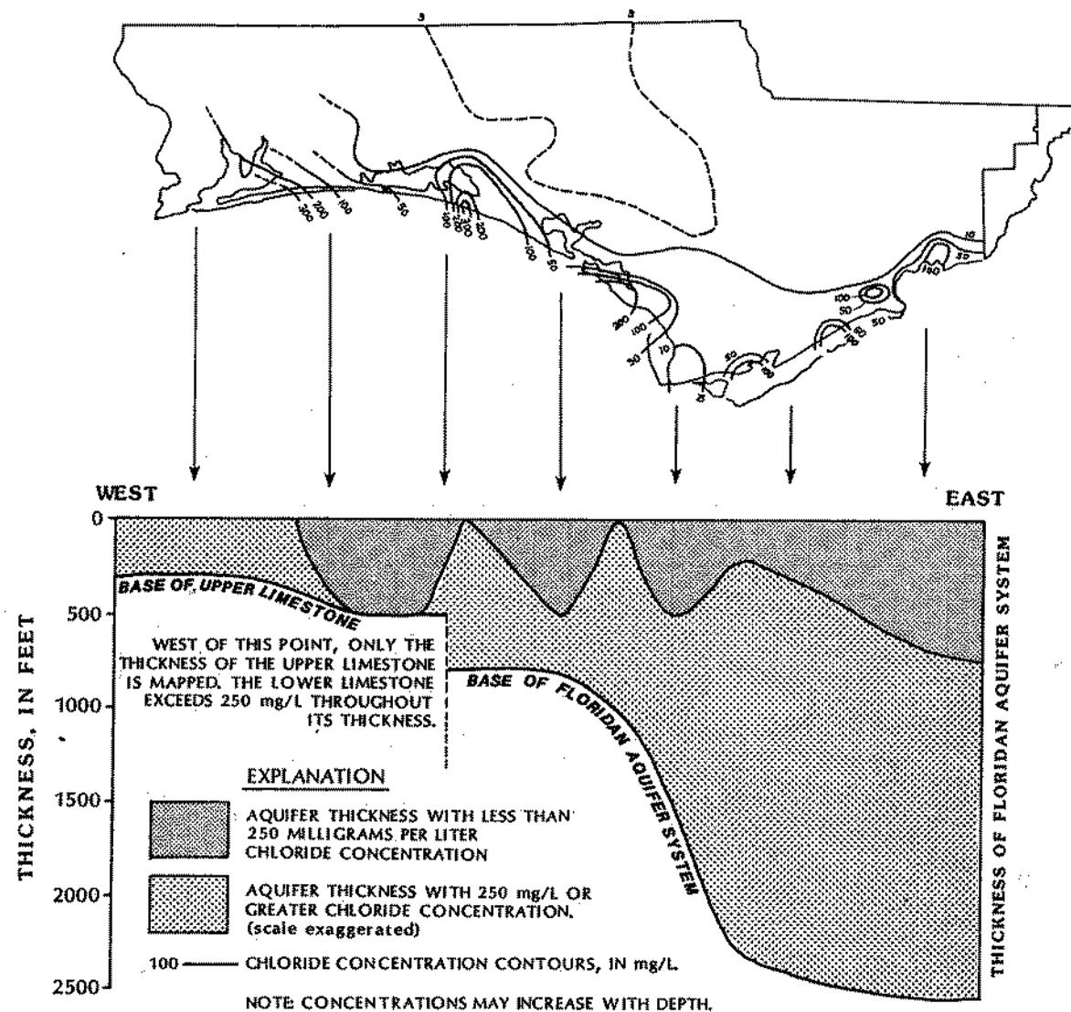
Figure 2. Profile of the Floridan Aquifer System and Ground Water Chloride Concentrations Along the Coast of Northwest Florida.
