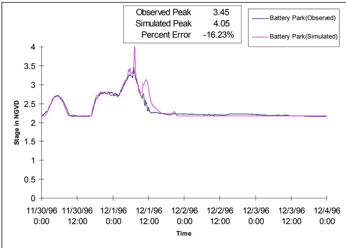
**Figure 45 -- Calibration Hydrograph for Battery Park**
