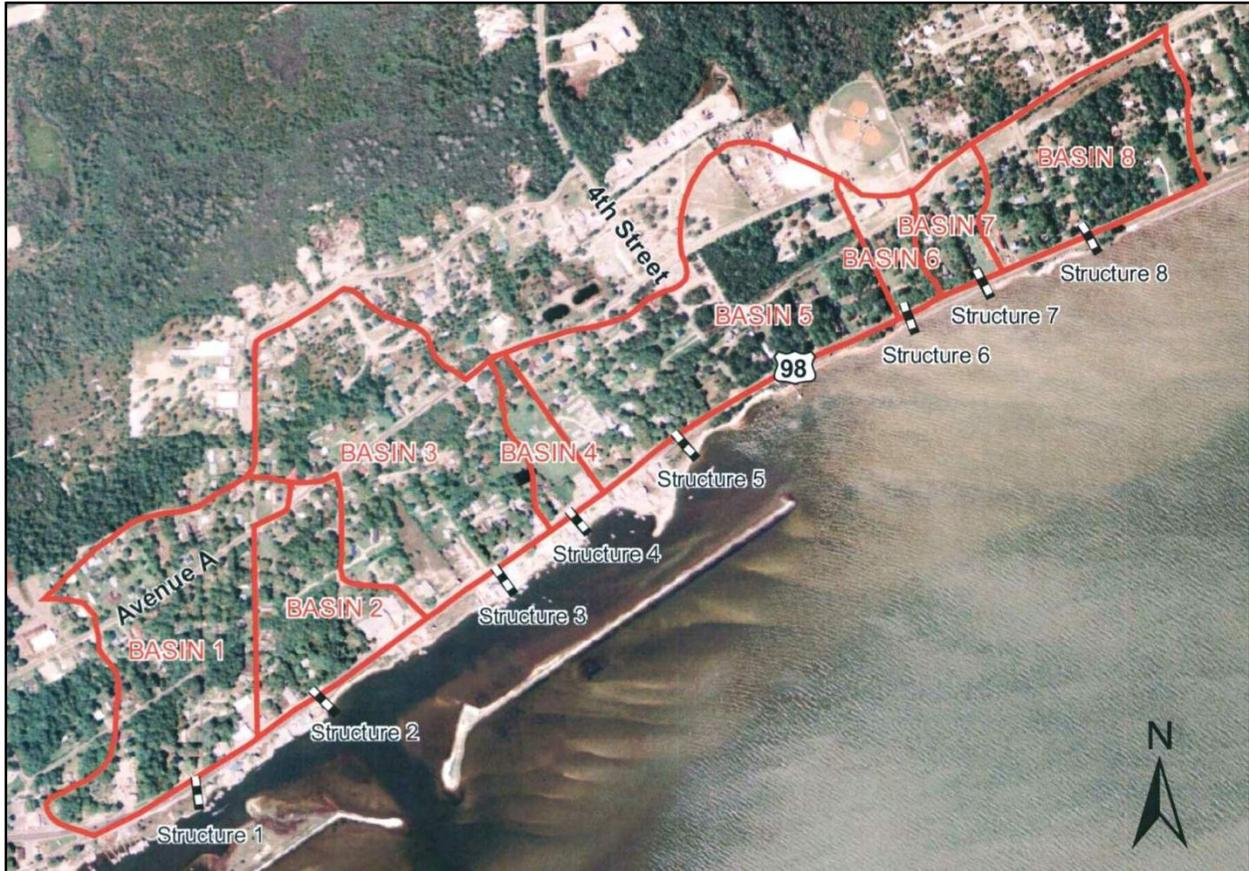
Figure 5: Avenue A Sub-basins and Outfall Structures
