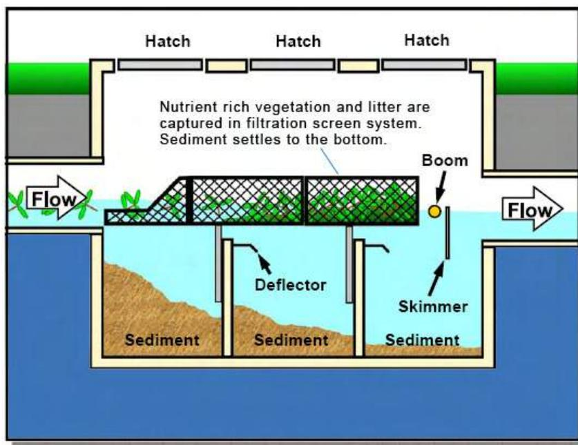
Figure 2: Schematic of a Baffle Box
