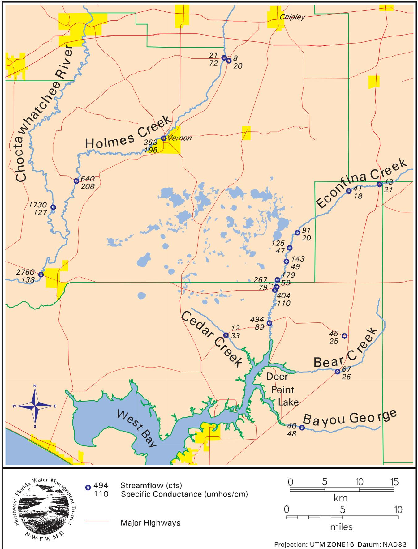
Figure 11. Measured Streamflows Used for Model Calibration, August 19 through August 22, 1996.
