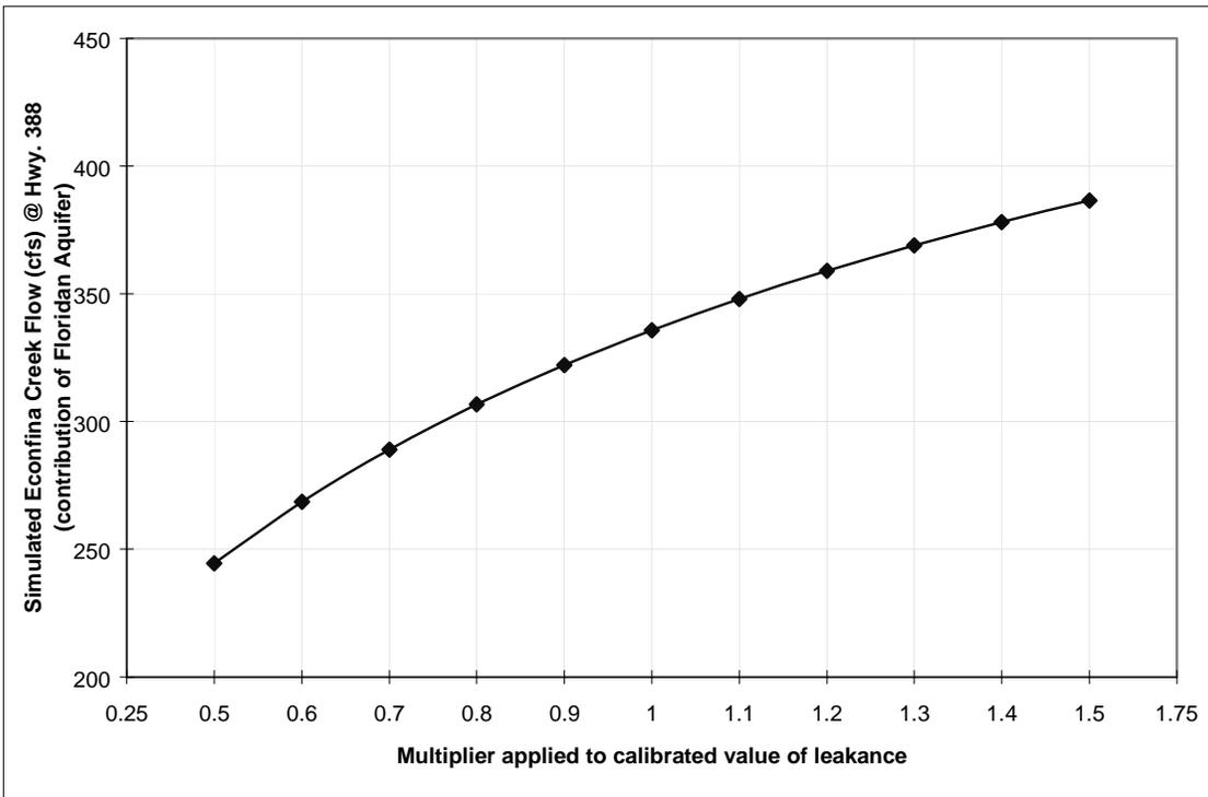
Figure 19. Sensitivity of Simulated Floridan Aquifer Discharge to Change in the Vertical Hydraulic Conductivity of the Intermediate System.
