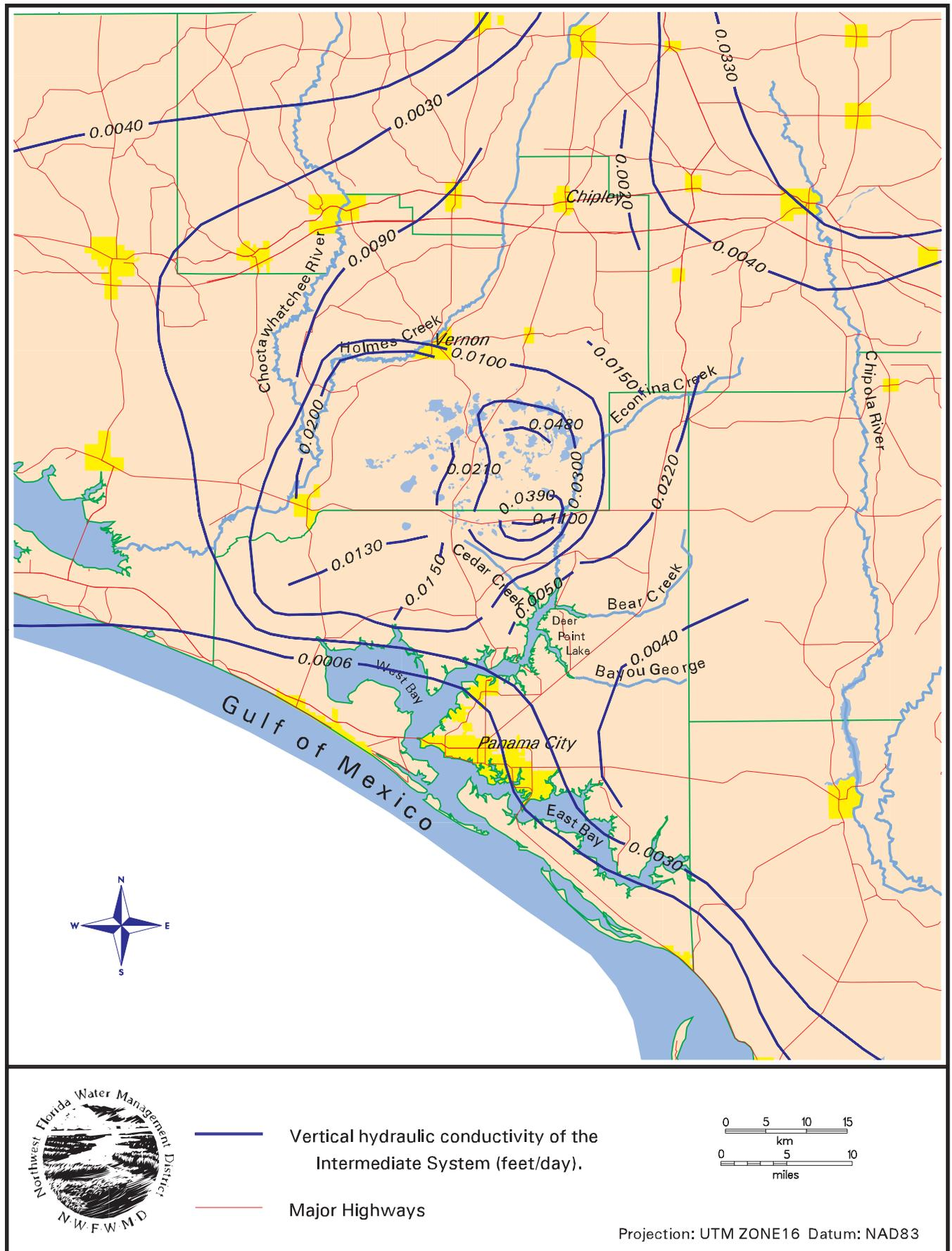
Figure 9. Vertical Hydraulic Conductivity of the Intermediate System as Used in the Model.
