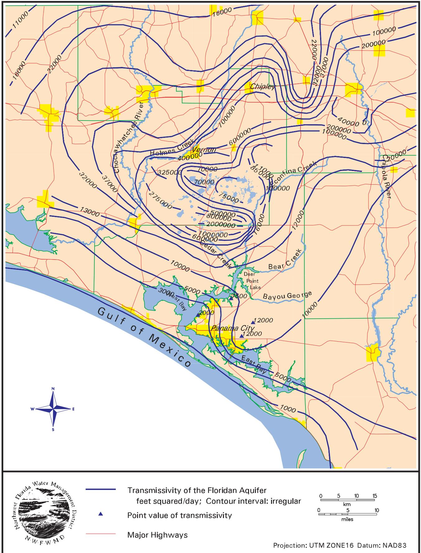
Figure 10. Transmissivity of the Floridan Aquifer System as Used in the Model.
