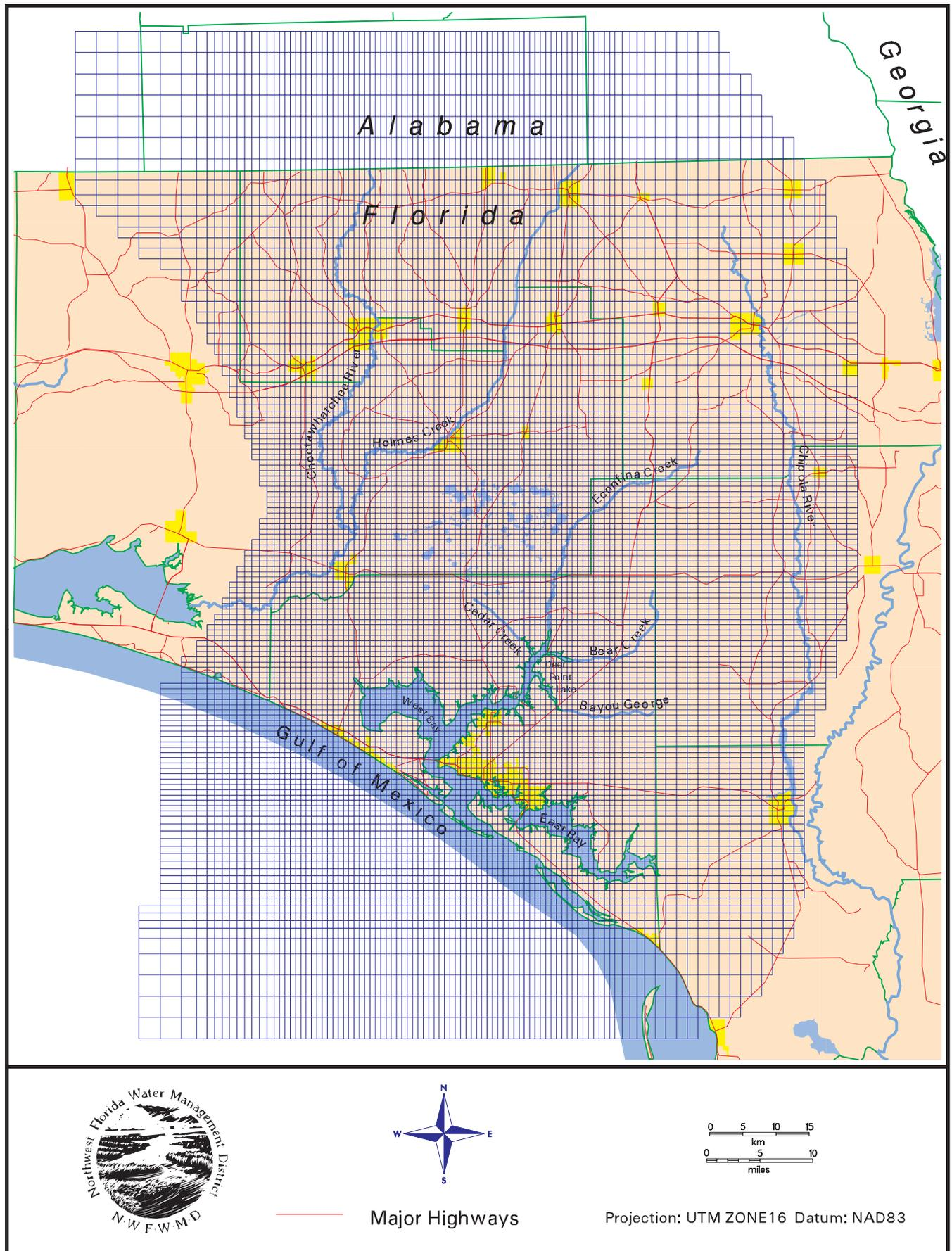
Figure 7. Model Grid as Used in the Regional Ground Water Flow Model.
