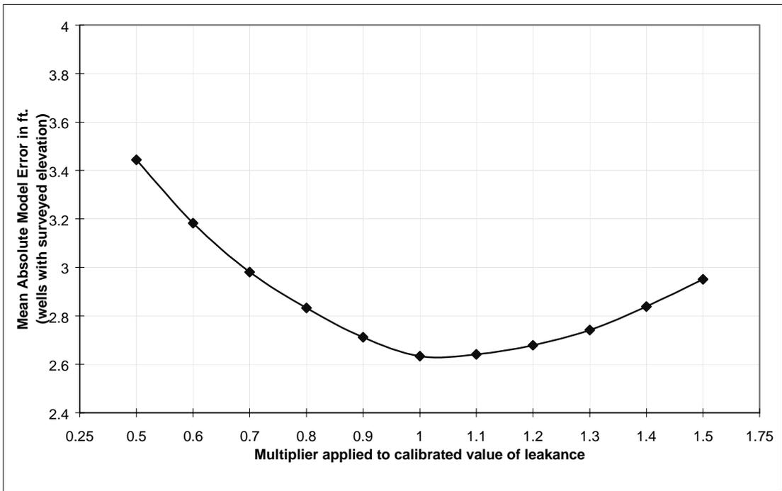
Figure 18. Sensitivity of Simulated Heads to Change in the Vertical Hydraulic Conductivity of the Intermediate System.
