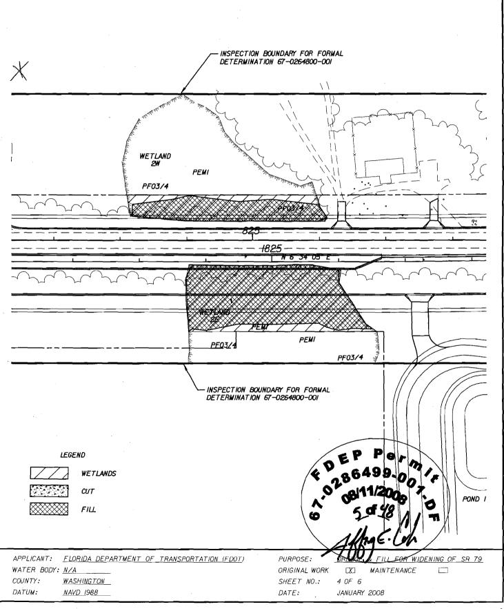
INSPECTION BOUNDARY FOR FORMAL DETERMINATION 67-0264800-001 EXISTING ROAD <del>1810</del> 1805 INSPECTION BOUNDARY FOR FORMAL DETERMINATION 67-0264800-001 LEGEND WETLANDS CUT FILL FOR WIDENING OF SR 79 PURPOSE: <u>FLORIDA DEPARTMENT OF TRANSPORTATION (FDOT)</u> APPLICANT: MAINTENANCE ORIGINAL WORK  $\boldsymbol{X}$ WATER BODY: N/A 3 OF 6 SHEET NO.; COUNTY: WASHINGTON\_ DATE: JANUARY 2008 DATUM: NAVD 1988
