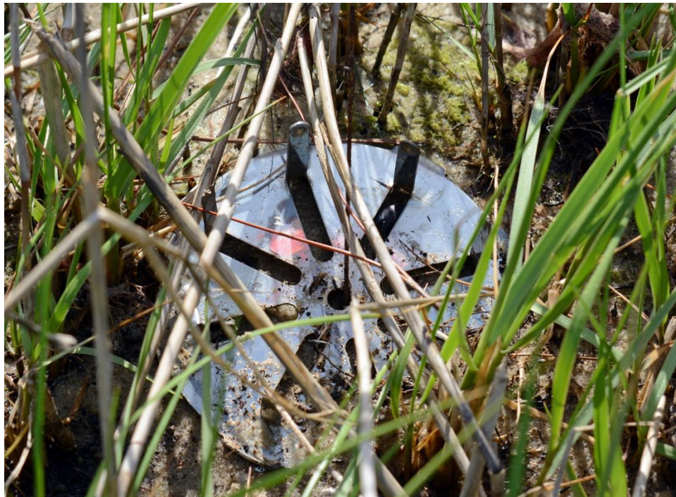
Figure 20. Reference Site Monitoring (Sediment Plate Exposed from Erosion) – 3/21/2022
