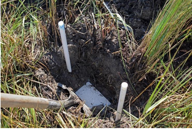
Figure 27. Installation of Additional Sediment Monitoring Points – 10/24/2022
