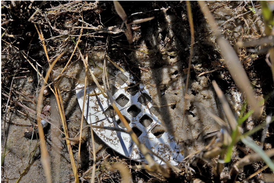
Figure 26. Initial Sediment Monitoring Plate (Plate A) Exposed by Erosion – 10/20/2022
