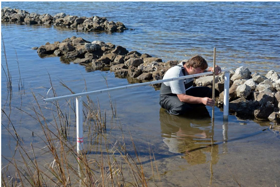
Figure 26. Sediment Accretion Monitoring Station (PVC Post Pairs) Between Breakwater and Shore (12/16/2024)
