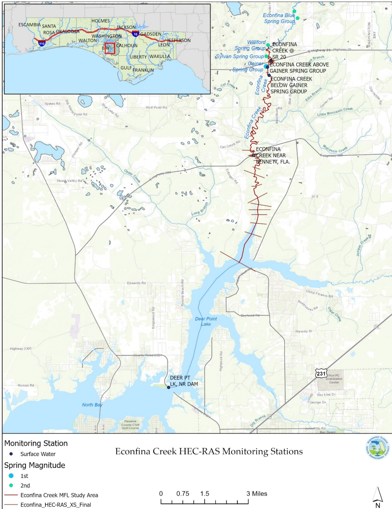
Figure 2-6. Econfina Creek Monitoring Stations Utilized to Develop Model Boundary Conditions
