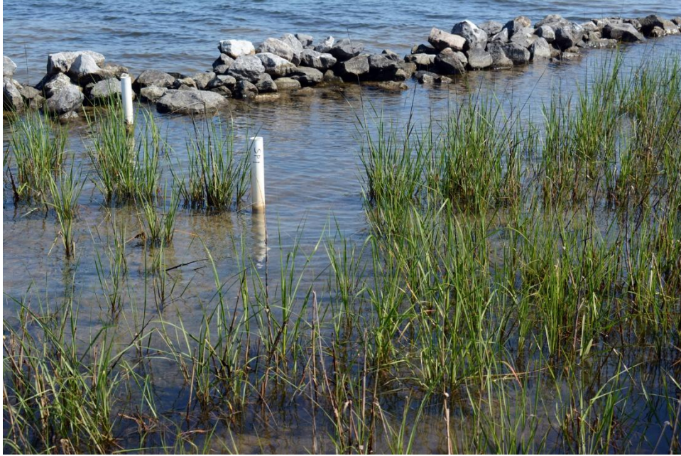
Figure 38. Sediment Accretion Monitoring Station (PVC Post Pairs; Station SP-1) and Marsh Expansion Between Breakwater and Shore (4/27/2026)
