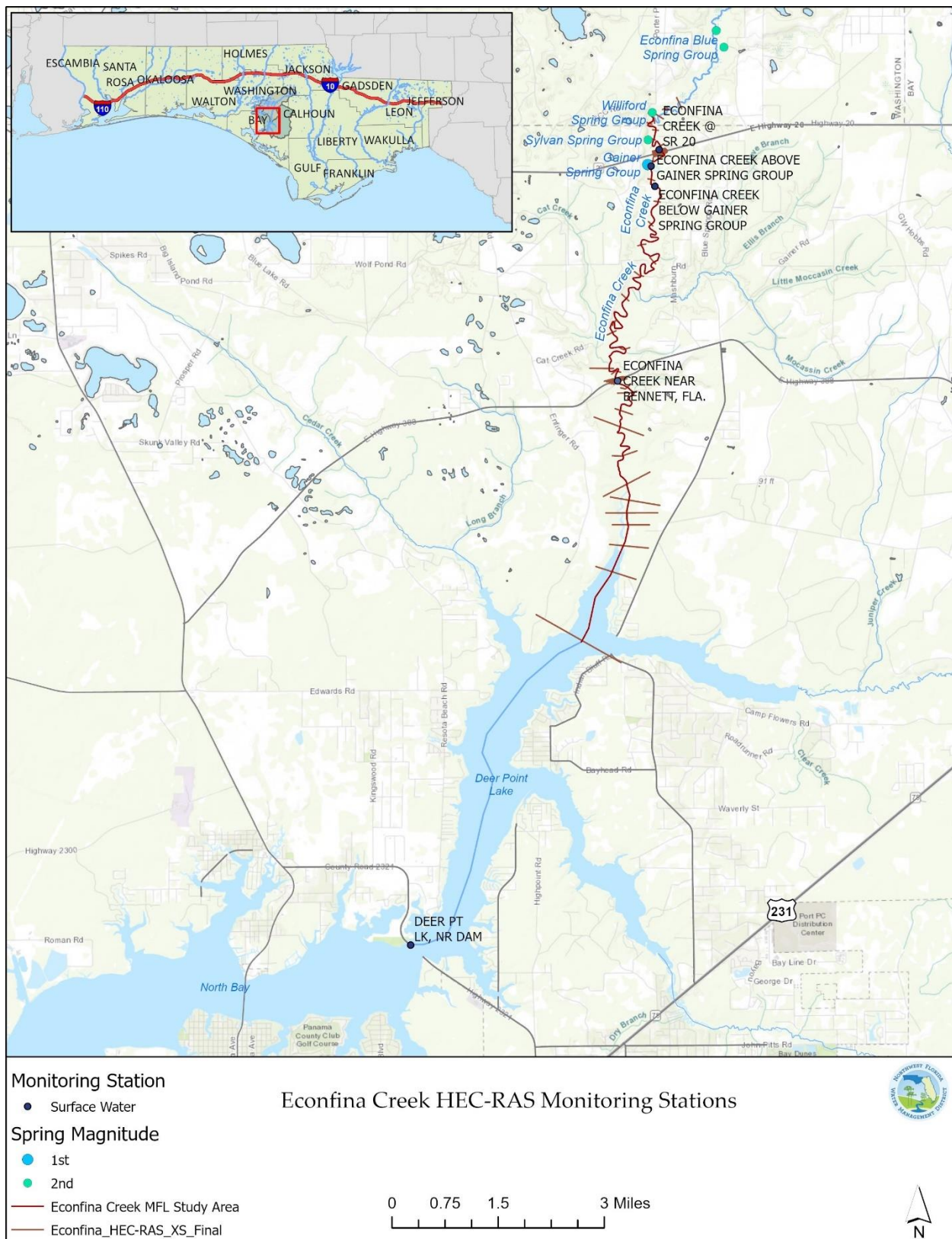
Figure 2-6. Econfinia Creek Monitoring Stations Utilized to Develop Model Boundary Conditions
